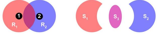
Fig. 2. (left) Sensing regions of two sensors 1 and 2.  $R_i$  is the sensing region of sensor  $i$ . (right) A partition of the overall sensing region  $R_1 \cup R_2$  into non-overlapping cells  $S_1, S_2$  and  $S_3$ , where  $S_1 = R_1 \setminus R_2$ ,  $S_2 = R_2 \setminus R_1$  and  $S_3 = R_1 \cap R_2$ .
