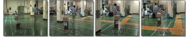
Fig. 5. A transporter robot. The person with a blue shirt is a target and a robot carries a yellow box.
