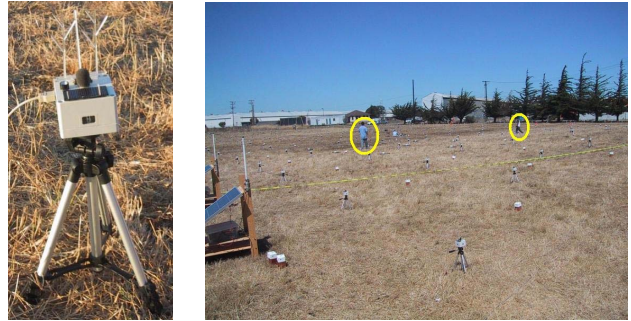
Fig. 1. Hardware for the sensor nodes. (left) Trio sensor node on a tripod. On top is the microphone, buzzer, solar panel, and user and reset buttons. On the sides are the windows for the passive infrared sensors. (right) A live picture from the 2 target pursuit-evasion game experiment. The targets are circled in yellow.
