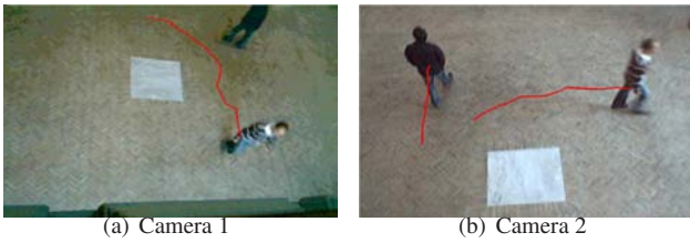
Figure 2. Track formation: formation of tracks based on object motion in two separate cameras.
