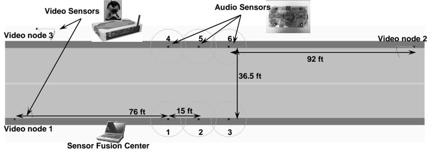
Fig. 4. Experimental setup
